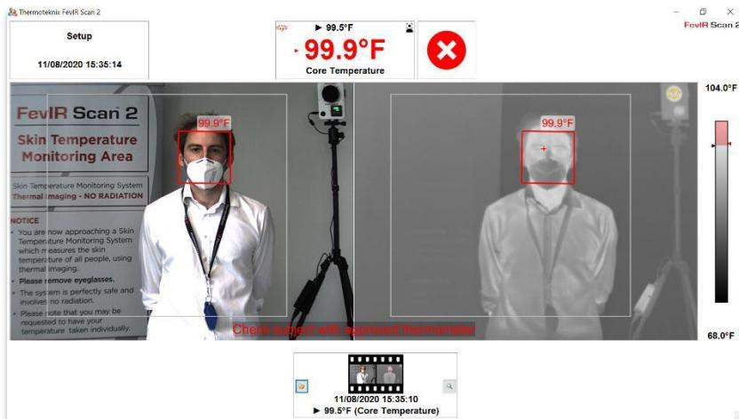
The alarm information is displayed at the top, and any temperatures on the thermal image measured above the alarm value will be coloured red. The actual temperature is shown in a red box adjacent to the subject’s face and will move with them as they move position within the scene.
